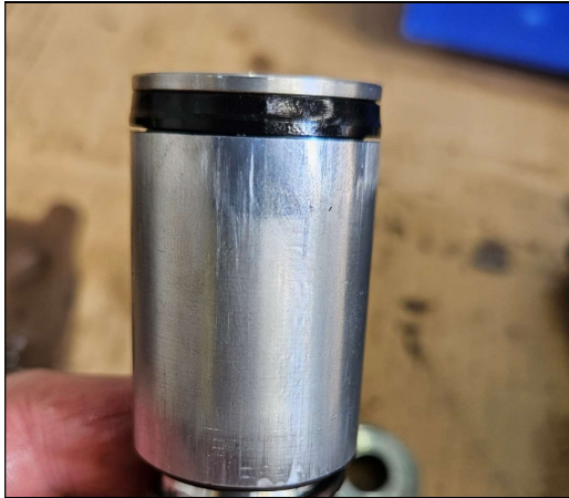
Figure 1: Hydraulic piston assembly scuffing
