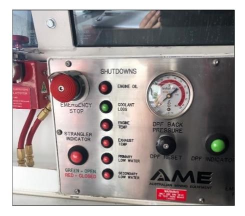
• An alternate improved fuel shut-off valve is registered refer part number 7-180412-751. Time to shut-down via this manual fuel shut-off valve is considerably reduced from the original shut-down valve.
