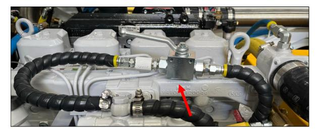
An improved low engine oil pilot valve (previously described in Bulletin 36138) is now design registered for use with MDR 114056 DES-7a. The improved oil valve shuts the engine down at a higher oil pressure than the original valve, providing a higher level of protection against engine failure due to low oil pressure.
