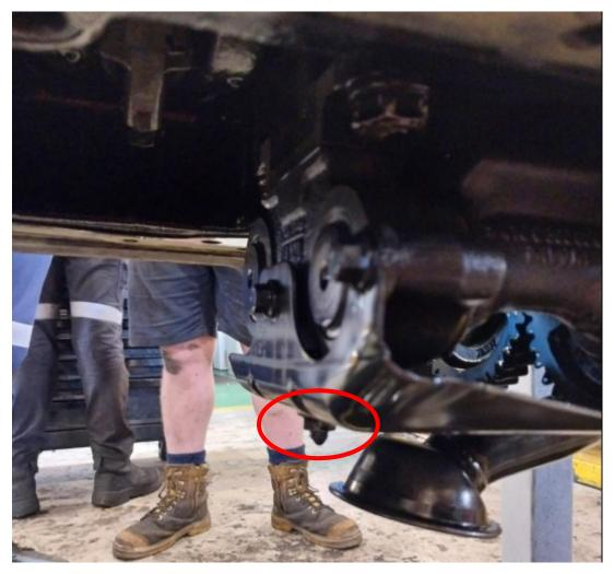
Figure 3: Deflector design 2 as installed with sump removed. Note protruding vertical fastener.
