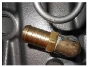
Figure 1 – 3/8 BSP elbow installed in the drivers side of the engine block In some cases an alternate drilled square fitting has been installed as per the below Figure 2
