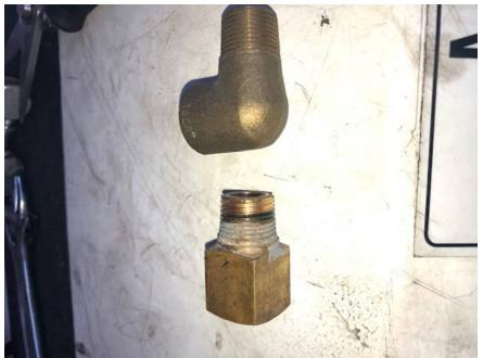
Figure 3 – Correct BSPT elbow (top) and Incorrect fitting (bottom)
