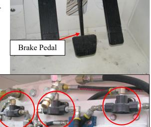
The front and rear service brake pressure gauges indicate the pressure in the lines to the relevant brake packs. Pressures will rise when the brake pedal is pressed. Design pressure for braking is 100psi.
