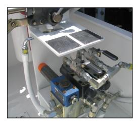
Cougar IME recommend that the pilot valves be scheduled for change-out at intervals of two years or 4000 hours operation.
