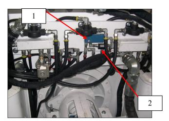
The declutch cylinder is piloted off (clutch engaged) when the park brake hold off pressure is above 240kPa.
