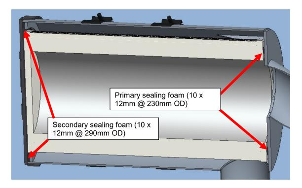
Figure 2: Sectional view of single filter arrangement depicting seal locations
